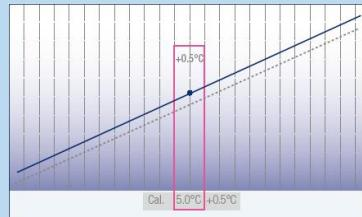
1-point calibration for compensation between the display temperature and the actual internal temperature
