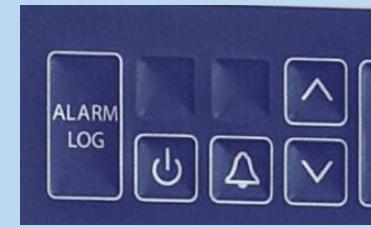
Min./max. temperature memory; last three temperature alarm and power failure events are saved
