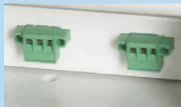
Volt-free contact and RS 485 serial interface for external temperature and alarm documentation
