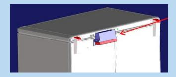
Reinforced lid hinges (as on GTL chest freezers) ensure high stability for frequent lid opening and closing
