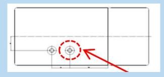
An access port (Ø 17mm) for an external temperature probe is provided in the base, 120 mm from the defrost water drain
